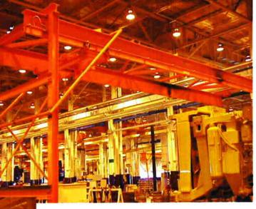
The gantry legs can be either ASCE rail supported or the legs can ride on pneumatics wheels.
